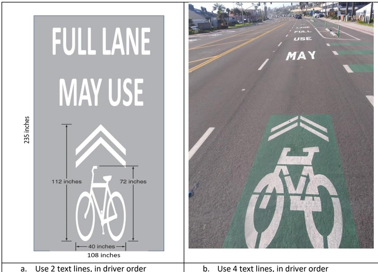
I would leave it to someone with Traffic Engineering expertise to determine the correct dimensions, spacing and the stretching of the letters for optimal readability as motorists drive over this augmented sharrow.
